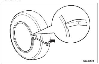
Wrap the tip of the bar with a cloth, insert it deeply into the notch provided in the wheel cover, and pry the cover away from the wheel.
